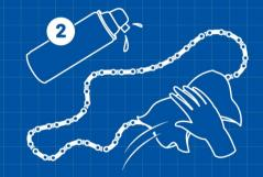
Grab the WD-40 Specialist, Chain Lube and spray onto the inner side of the chain, and manually spin the rear tyre as you spray. Wipe access away with clean cloth.
