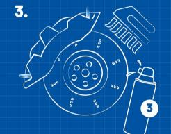
Remove gunk and grimes on the brake calipers, without dismantling using the WD-40 Specialist Brake & Parts Cleaner.
