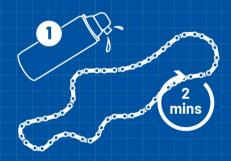
Degrease the chain, spray a generous amount of WD-40 Specialist. Machine & Engine Degreaser, let is sit for 2-3 mins and wipe away.
